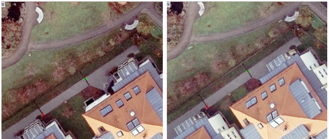
Fig. 117. The left image shows triplet point, located in the center of triple overlap area, the right one – triplet point from the right image
