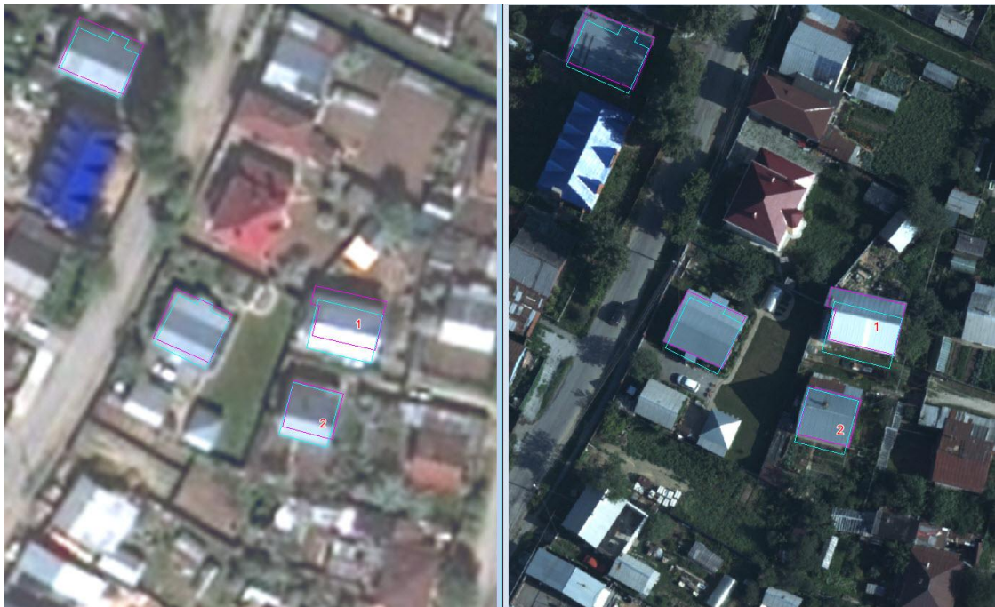
Figure 4 - The prominent part of 1.5 m wide(1) is not represented, the form (shape) and size of the building are represented with an accuracy error of 2 m (2).
