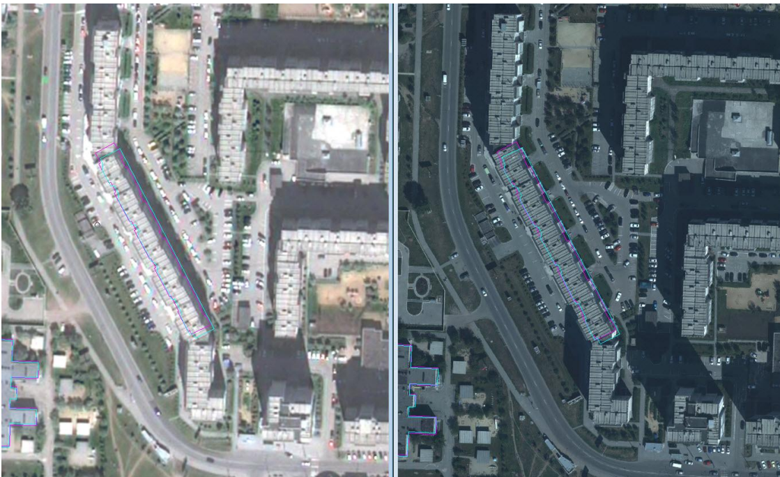
Figure 6 - Architectural figured details can be omitted (the prominent parts on the left-hand side of the building are shown, those on the right-hand side are omitted).
