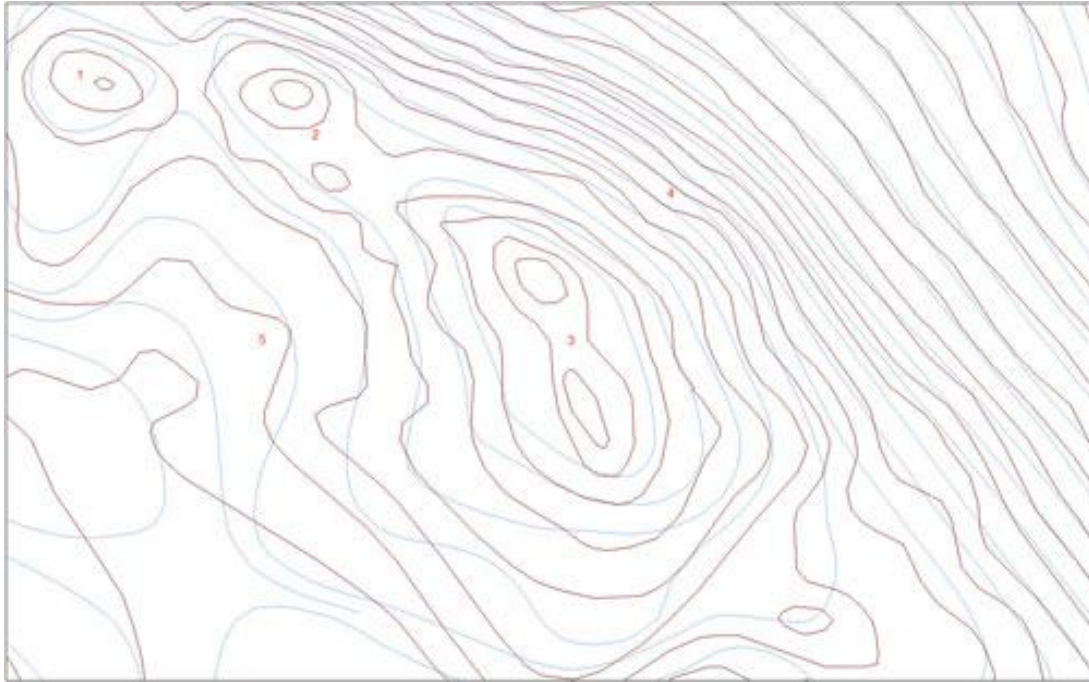
Figure 9 - Comparison of the contour lines: brown — based on the aerial photographs, blue — based on the Pleiades image. Hills ( up to 3-4 m high) (1), (2), (3) are omitted, the ravine (4), (5) is not represented.
