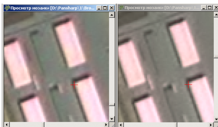
Fig. 72. Pan sharpening operation result by Broyer method without color correction (left) and using neighbor color correction (right)
