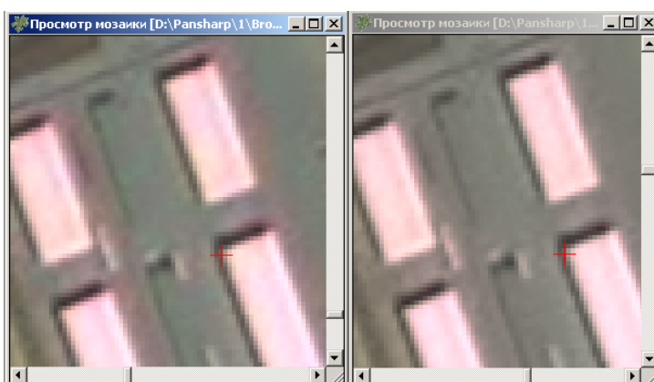
Fig. 84. Pan sharpening operation result by Brovey method without color correction (left) and using neighbor color correction (right)
