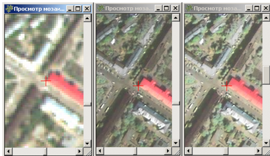
Fig. 79. Initial color image (left), pan sharpening operation result by Brovey method without color correction (in center), with automatic correction (right)
