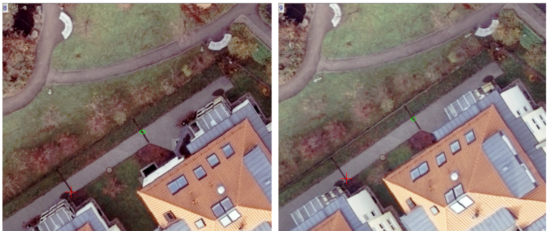
Fig. 114. The left image shows triplet point, located in the center of triple overlap area, the right one – triplet point from the right image
