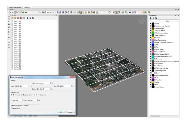
Fig. 10. The Splitting sheets displaying
