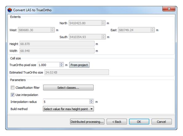
Fig. 20. The Convert LAS to True Ortho window
