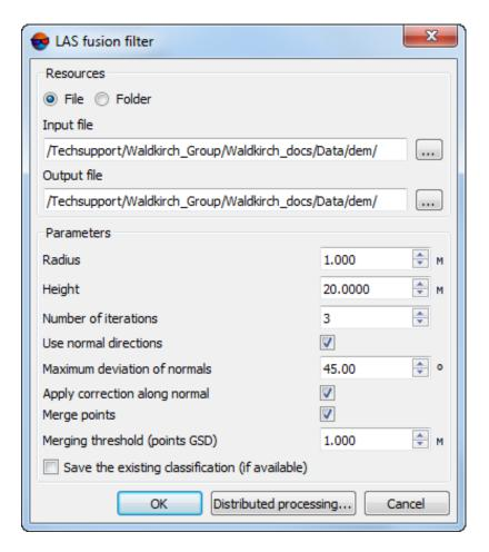
Fig. 40. The LAS filtering window
