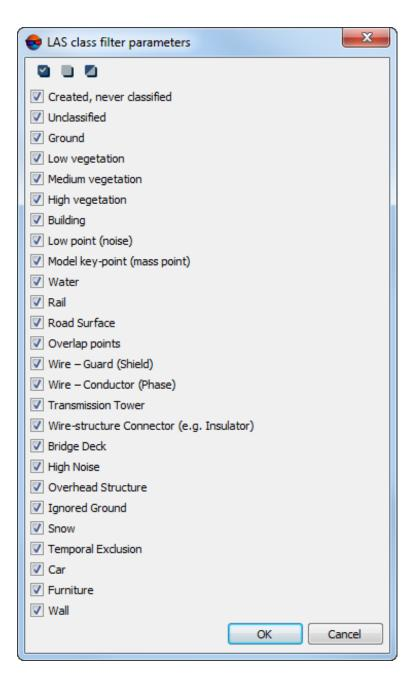
Fig. 35. The LAS classification filter parameters window
